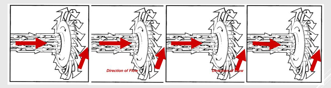
Placing impellers in series increases the amount of head produced
