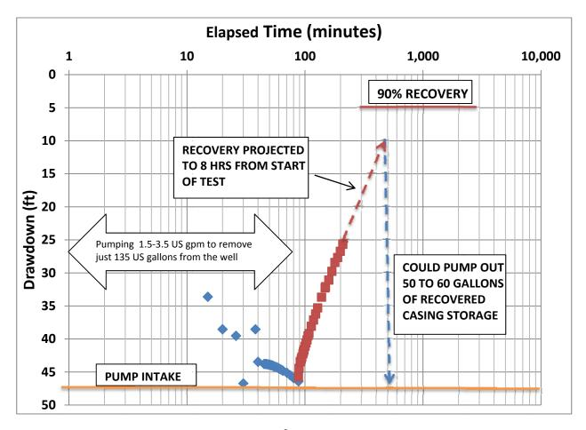
**Example 4 – Example Semi-Log Graph for Plotting Drawdown and Recovery Water Levels**
