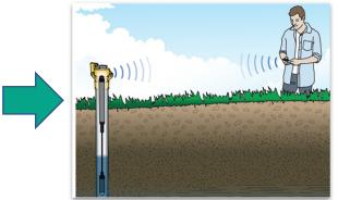
Install & maintain groundwater level data loggers to collect hourly water level measurements
